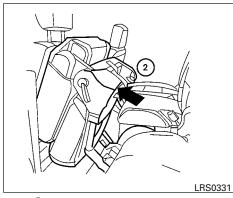
Then (2) lift up on the lower corner of the seat base and tip the outboard seating position of the 2nd row bench seat forward. To exit the 3rd row bench seat, lift up on the same seatback latch and fold the seatback forward onto the seat base. Then lift up on the seat base and tip it forward.
